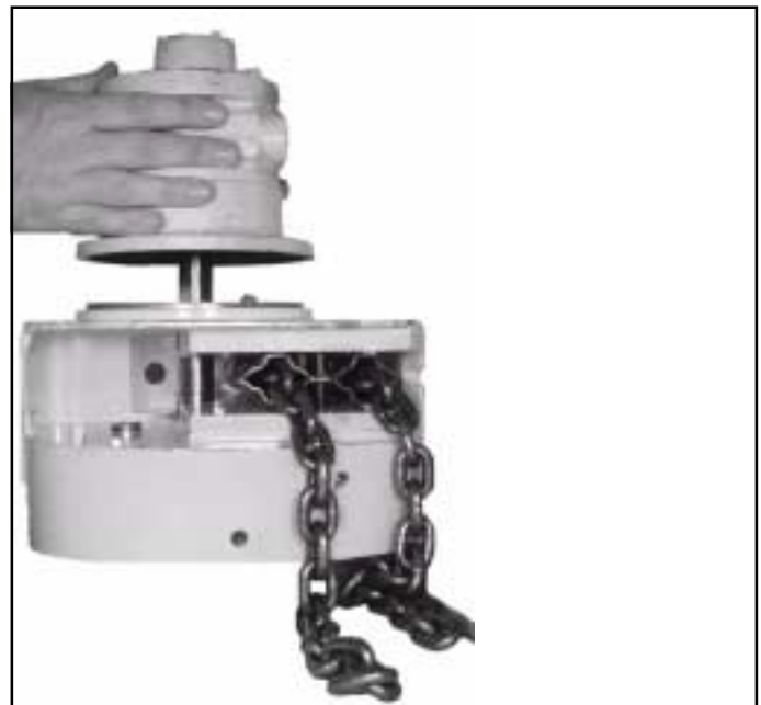
Figure 7-8. Removing Motor Assembly
