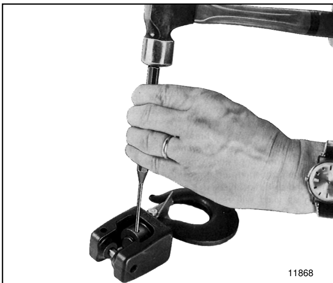
Figure 7-23. Removing Roll Pin Securing Hook Nut to Hook Shank
