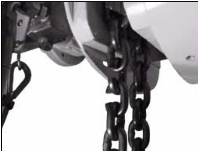
Figure 5-4. Installing Coil Load Chain Using Two "C" Links (single line of load chain.)
